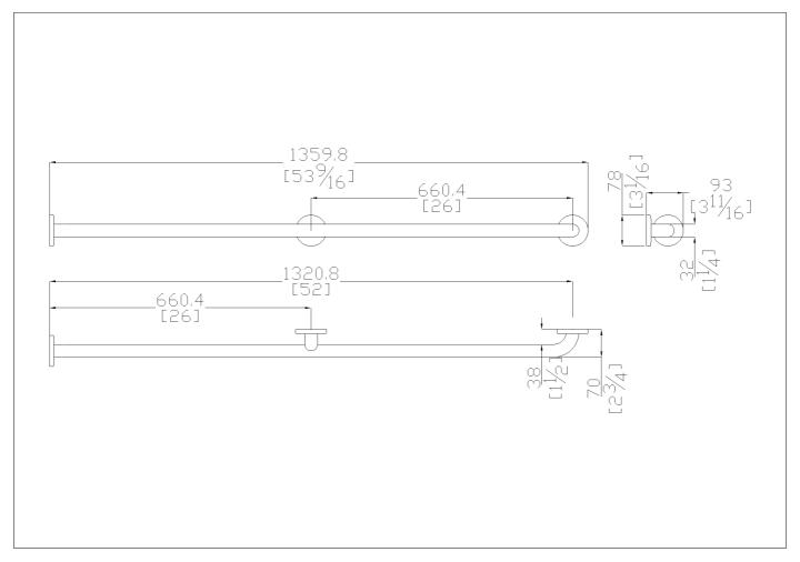
Safety grab bar, straight, wall to floor, with 3 wall brackets, made of seamless stainless steel AISI 304 pipe, with satin finish
