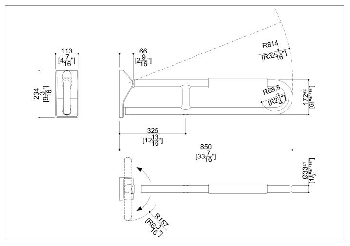
Folding and rotating grab bar, equipped with arm rest, ø 33 mm made of seamless zinc-plated steel pipe, coated with antimicrobial, biocompatible and warm-to-the-touch vinyl
