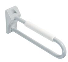
Folding and rotating grab bar, equipped with arm rest,  $\emptyset$  33 mm made of seamless zinc-plated steel pipe, coated with antimicrobial, biocompatible and warm-to-the-touch vinyl
